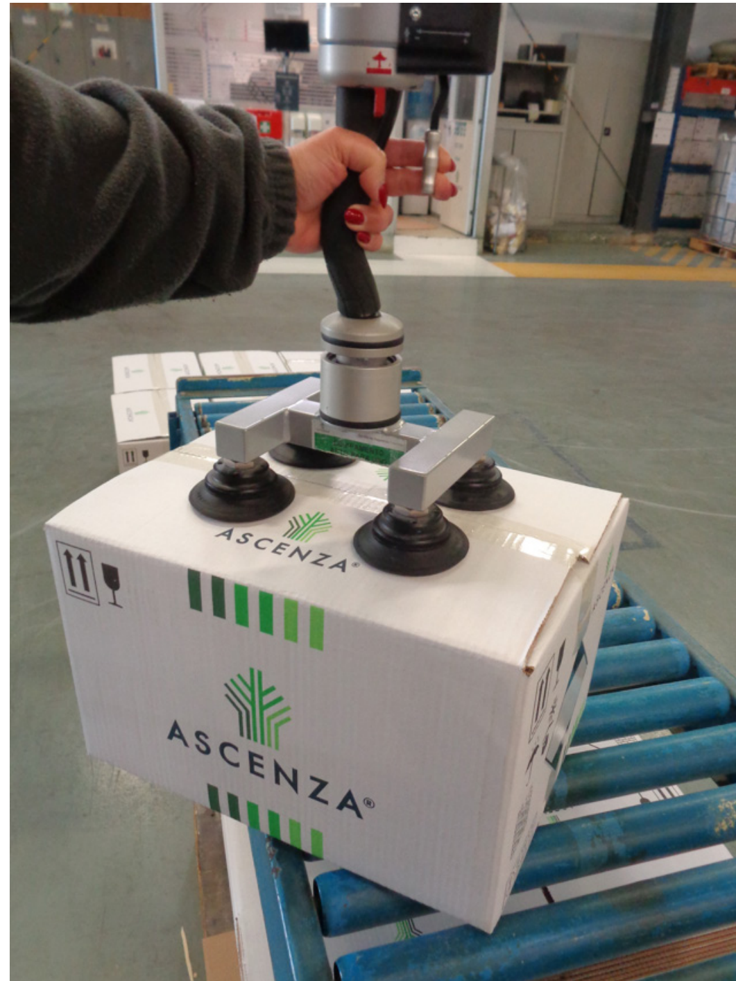
Vacuum tubes supporting a box at Ascenza industrial plant, in Setúbal, Portugal
